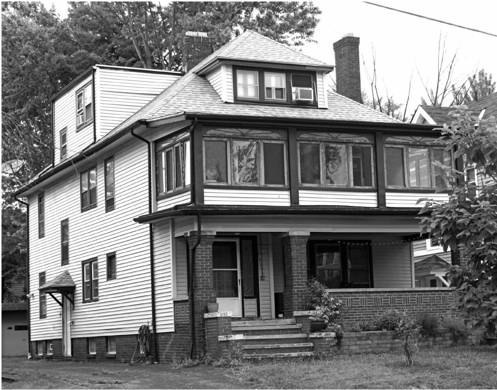
Figure xxxvii: 3165 Meadowbrook Blvd., what seems at casual glance a usual Type 1 triple, sports at least three special features: 1) five-light, fan-style transom windows topping the casement windows of the porch enclosure 2) Wrightesque perimeter grid windows (Figure lviii shows this better) 3) leaded-glass sidelights around front door (Figure xliii shows this better) (Peskin, L.).
